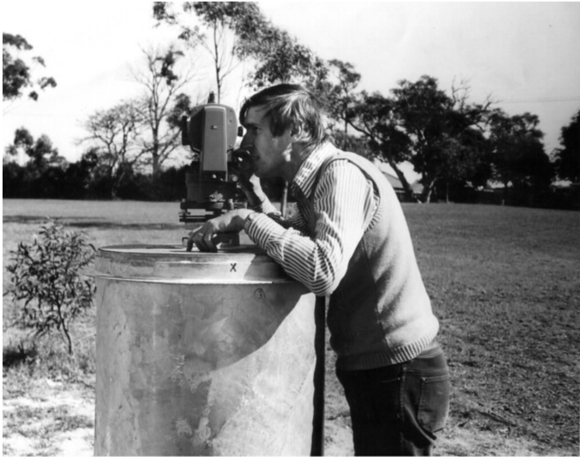
Measurement of the EDM Calibration Baseline of the National Measurement Laboratory, CSIRO, Lindfield, Sydney J. M. Rüeger with a Hewlett-Pakard HP3820A electronic tachometer on one of the pillars, 23.4. or 8.5.1981 Photo by CSIRO, Scanning by J. M. Rüeger Personal Collection of J. M. Rüeger) (Item 1981-01-01)
