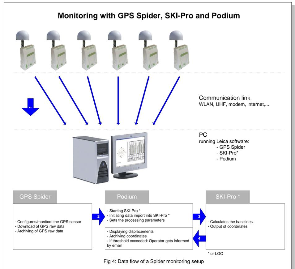
Fig 4: Data flow of a Spider monitoring setup
