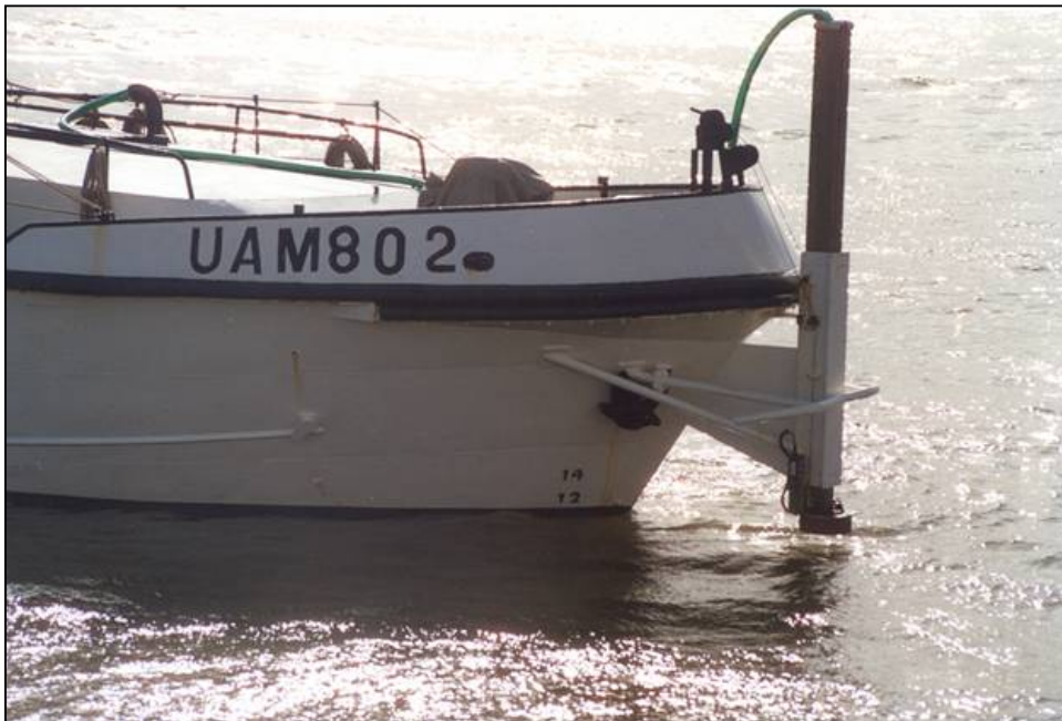
Fig. 3.19 "Transducer installation over the bow"
