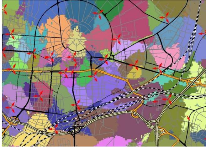
Figure 6: Exemplary mobile phone network with cells and antenna locations and orientations
