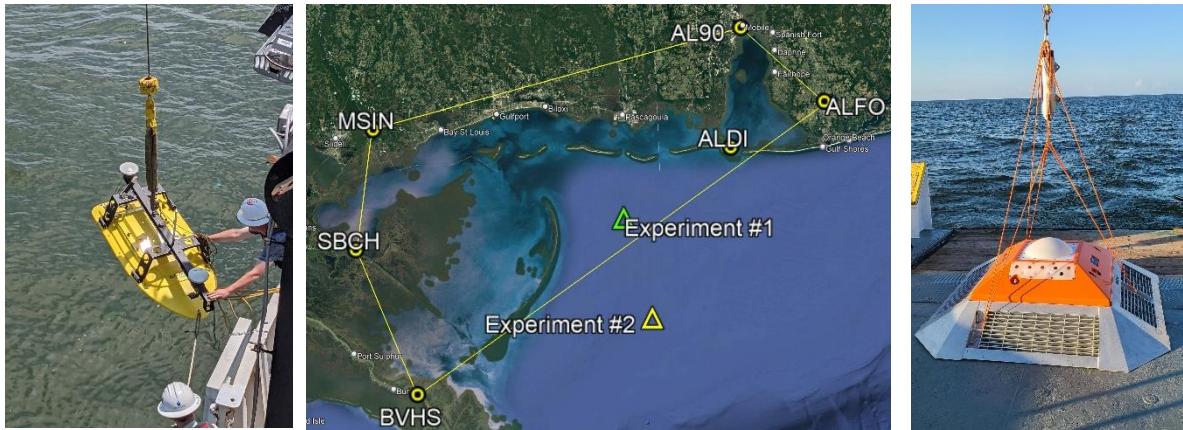
Figure 2 Left panel: EchoBoat deployment. Center panel: experiment #1 and #2 locations: 52.4 and 78.6 km from the nearest CORS (ALDI). PCLA, DSTN, and PNMA (are towards the east but not shown); they enclosed location #2 in the CORS network. Right panel: Bottom package deployment.
