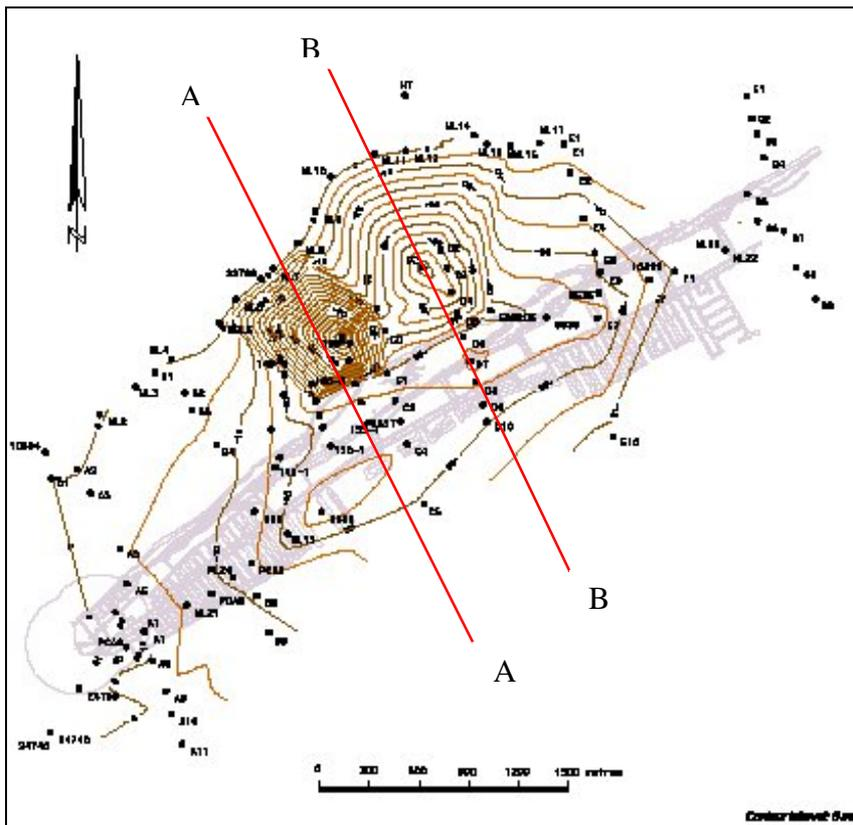
Figure 2. Mine layout and the subsidence isolines (2002).
