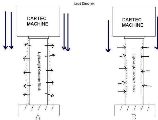
Dot Line is Deformation Direction of Lightweight Concrete during the axial compression testing in progress.
