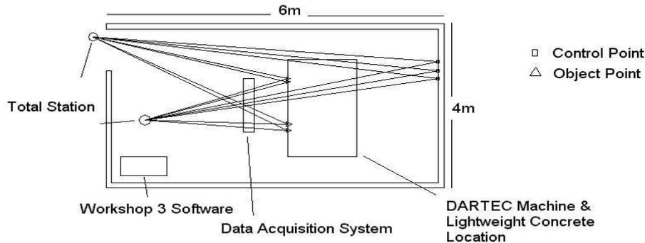
Figure 3: Sketch of the geodetic deformation network established in the laboratory
