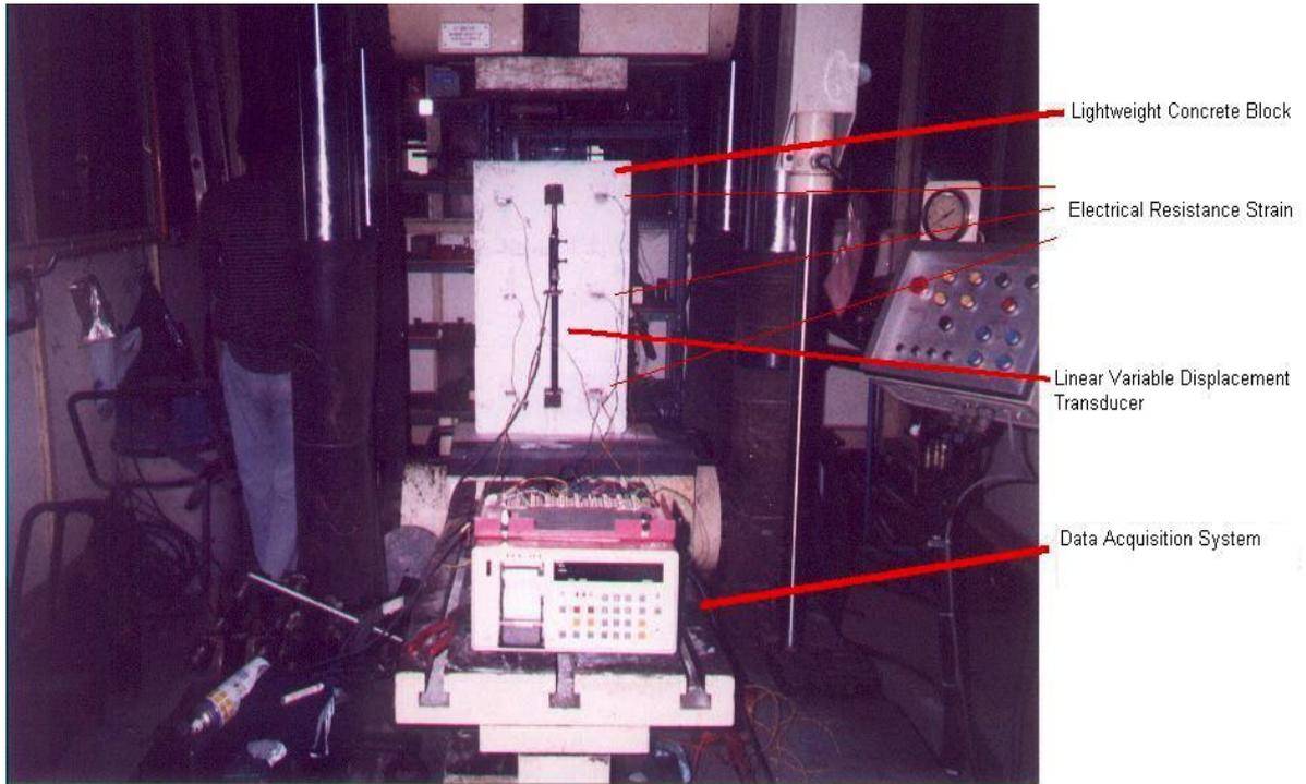
Figure 5: The set-up of Non-Geodetic Instrumentations
