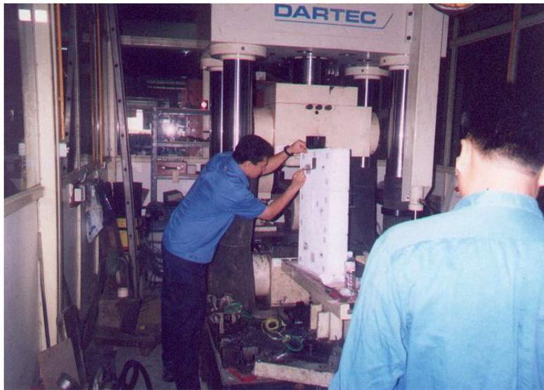
Figure 2: DARTEC Testing Machine
