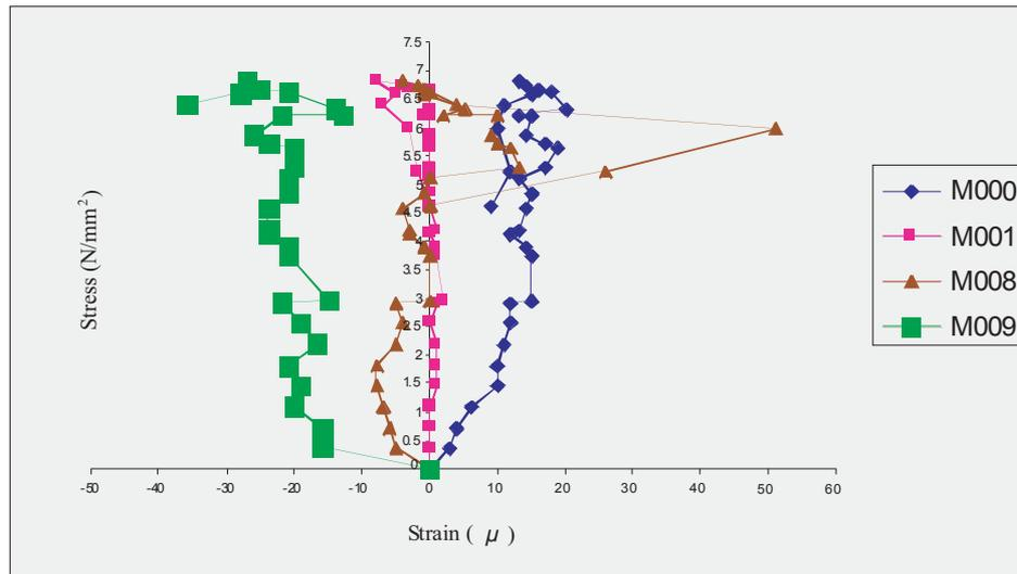
Figure 7: Strain-Stress relationship of the surface of lightweight concrete
