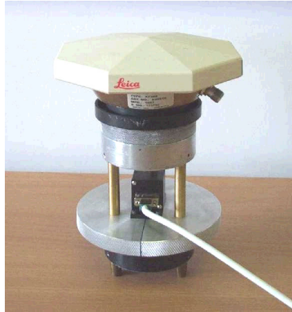
Fig. 11, The accelerometer and GPS antenna co-located
