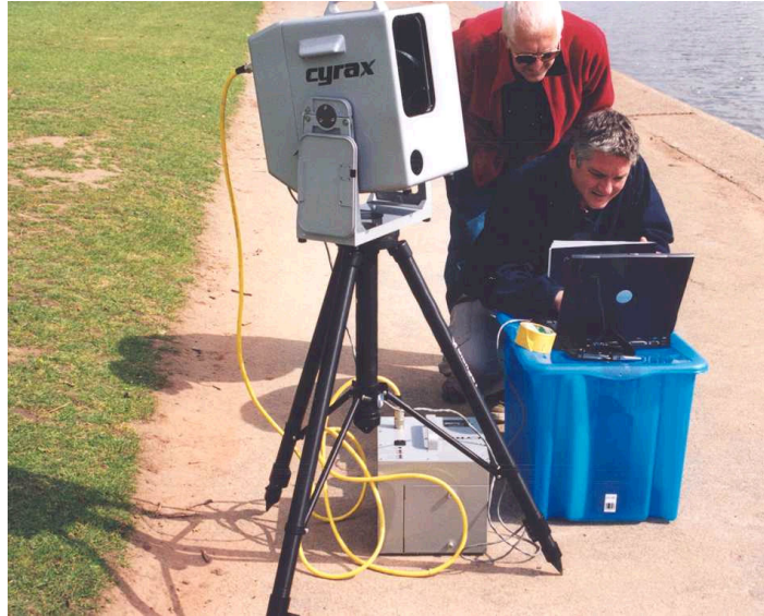
Fig. 6, A CyraX laser scanner being used to measure the dimensions of the bridge
