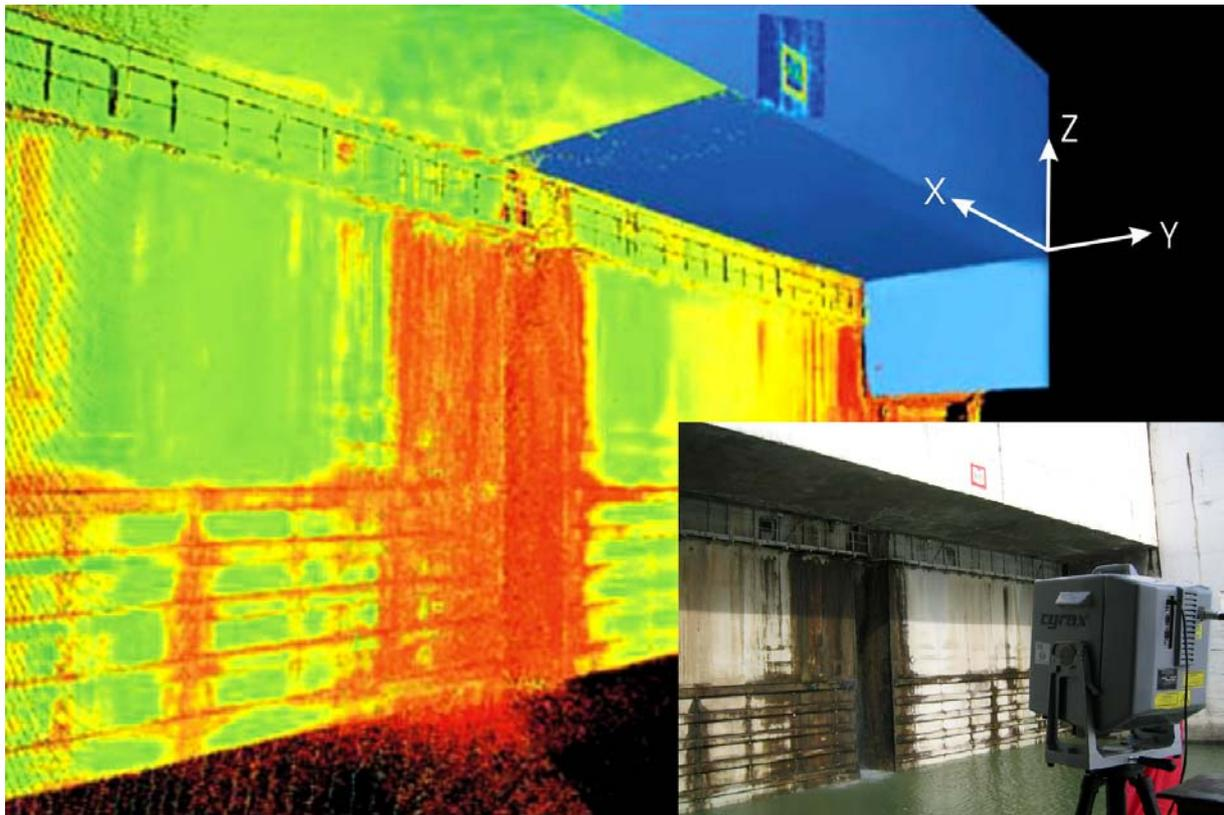
**Fig. 6:** The lock gates as point cloud viewed from the observation platform with the definition of a local reference frame using three perpendicular planes of the the rigid concrete walls.
