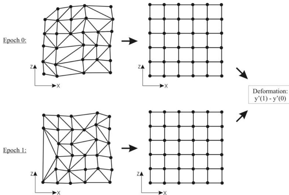
**Fig. 7:** Raw point clouds with an irregular and non-uniform sampling (left) and the interpolated grid (right) identical for every point cloud (epoch). The difference in y-direction represents the deformation.
