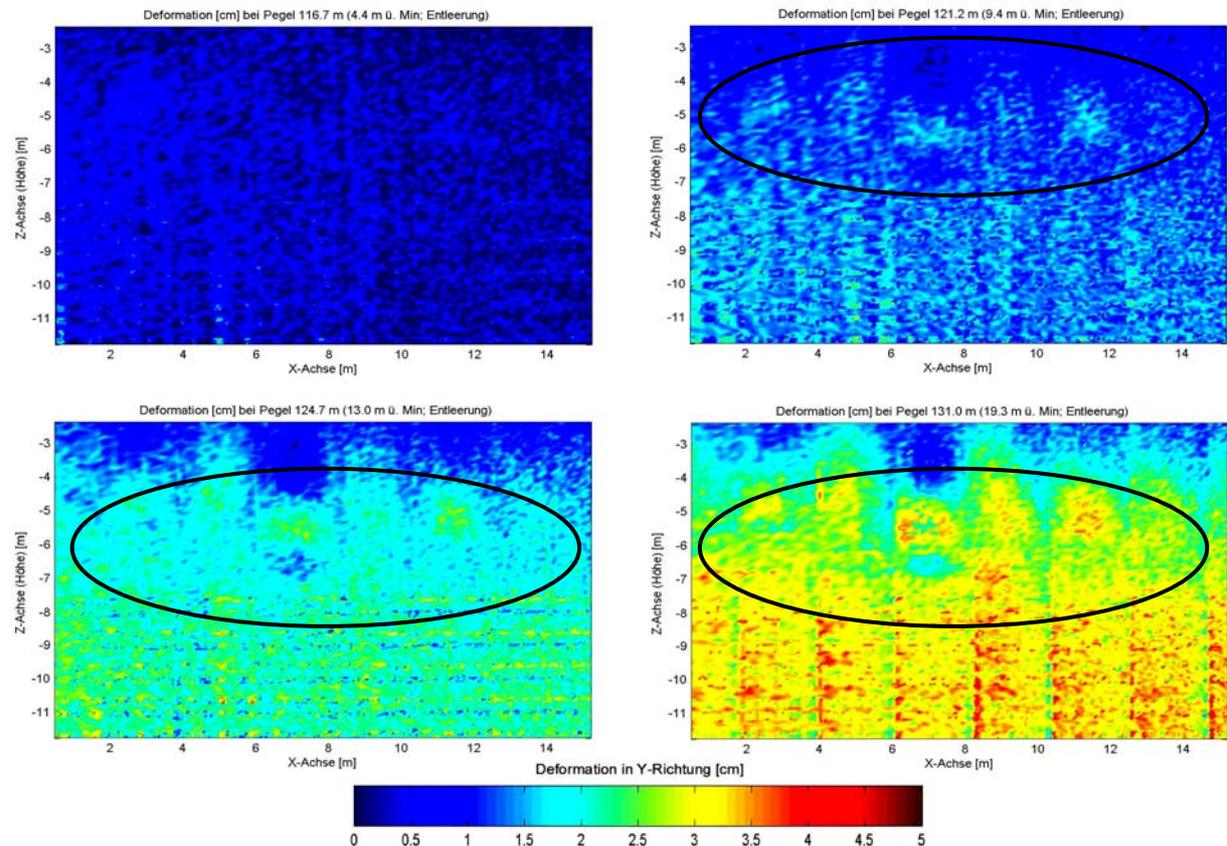
**Fig. 8:** Deformations observed at constant liquid levels of 4.4m (upper left), 9.4 m (upper right), 13.0 m (lower left) and 19.3 m (lower right).
