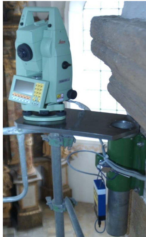
Fig. 1b: Total station with temperature sensor
