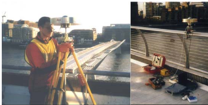
Figure 2 and 3: The Reference SR530 GPS receiver (left), and a GPS receiver and Kirstler Accelerometer (right)
