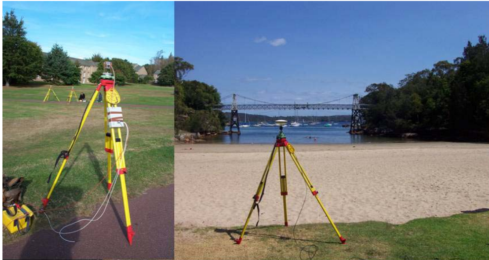
Figure 10: A GPS pseudolite being used during trials at the University of Nottingham (left) and Parsley Bay, Sydney, Australia (right)
