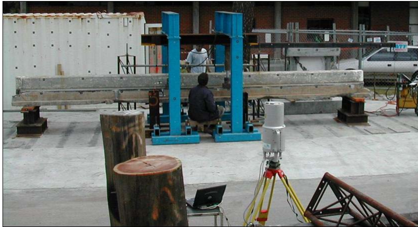
Fig. 1: Concrete beam and the Riegl LMS-Z210
