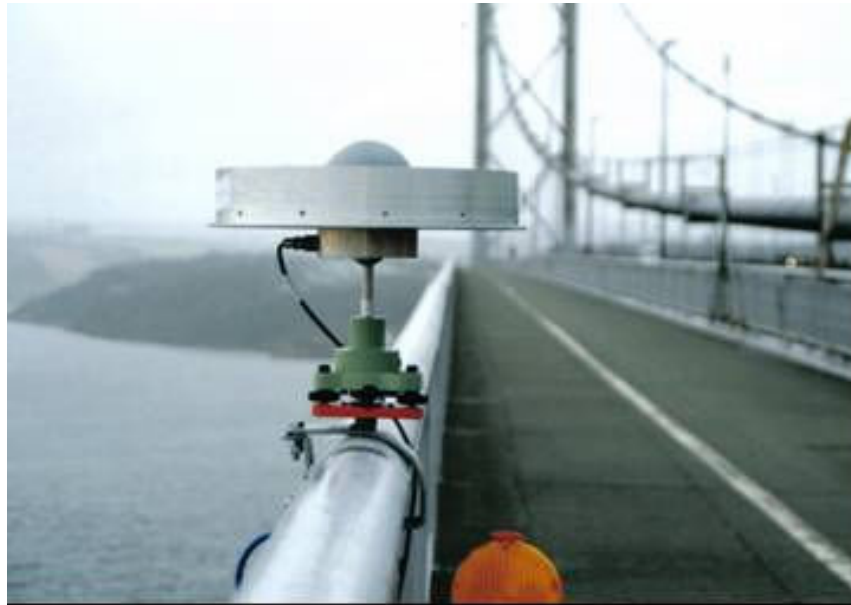
Figure 3. A Leica AT504 choke ring antenna clamped onto the bridge's handrail
