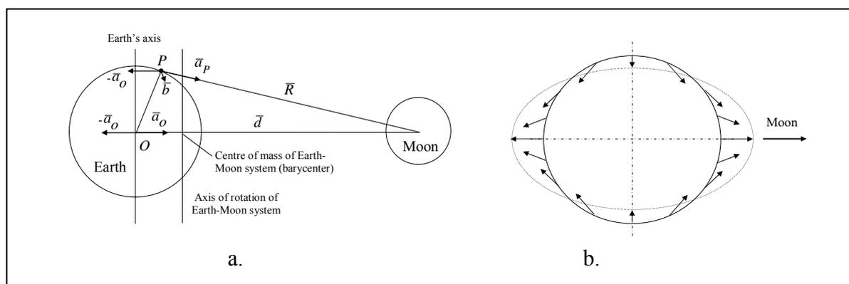
Figure 1: Definition of tidal acceleration (a), Tide-producing forces and deformation of the Earth (b)
