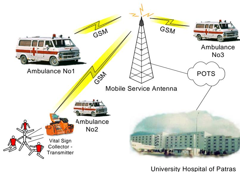
Fig 9. Overall architecture of the system developed.
