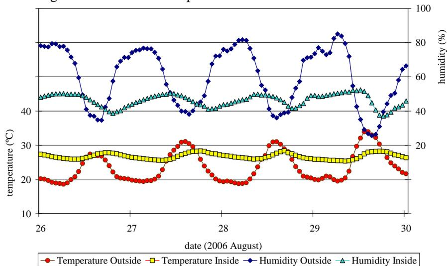
Fig. 10 – Temperature and humidity inside and outside the Pavilion (no events)
