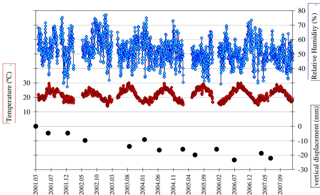
Fig. 17 – Temperature and relative humidity of the air and vertical displacements of B14
