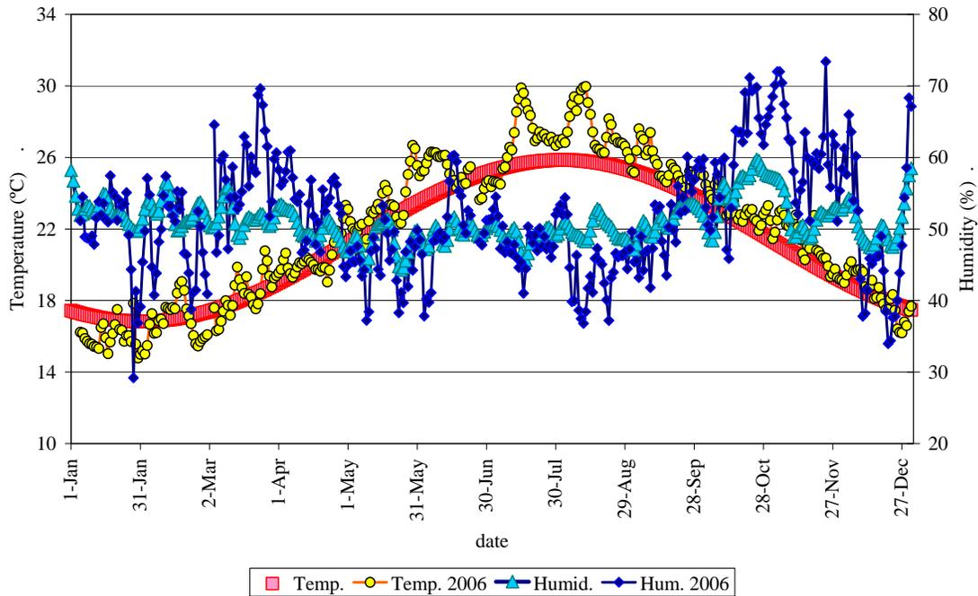
Fig. 18 - Temperature and relative humidity estimated and measured in the year 2006
