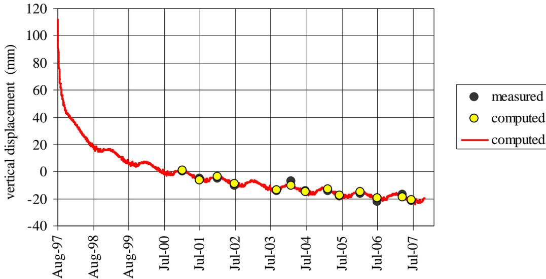
Fig. 19 – Measured and computed displacements
