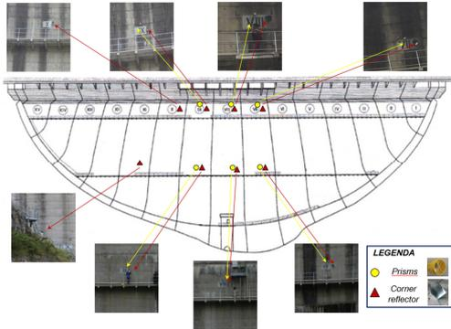
**Fig. 2** Location of prisms and corner reflector on the dam
