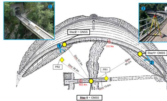
Fig. 1 Measurement network
