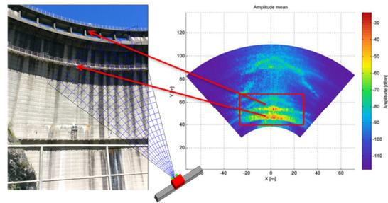
**Fig. 4** Mean amplitude obtained by averaging the all 7806 images. The red rectangle identifies the area of interest.
