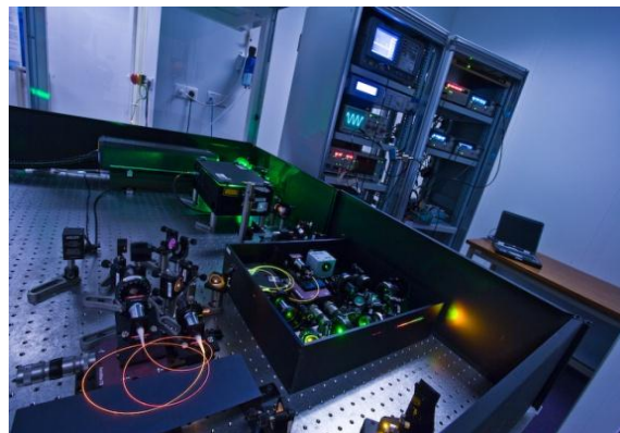
Fig.2 The VSL frequency comb in operation. The colored fibers broaden the spectrum that is emitted by the Ti:Sapphire laser over the full visible spectrum, which is used for optical frequency calibration. For distance measurement the original Ti:Sapphire spectrum is used, ranging from 810-830 nm.
