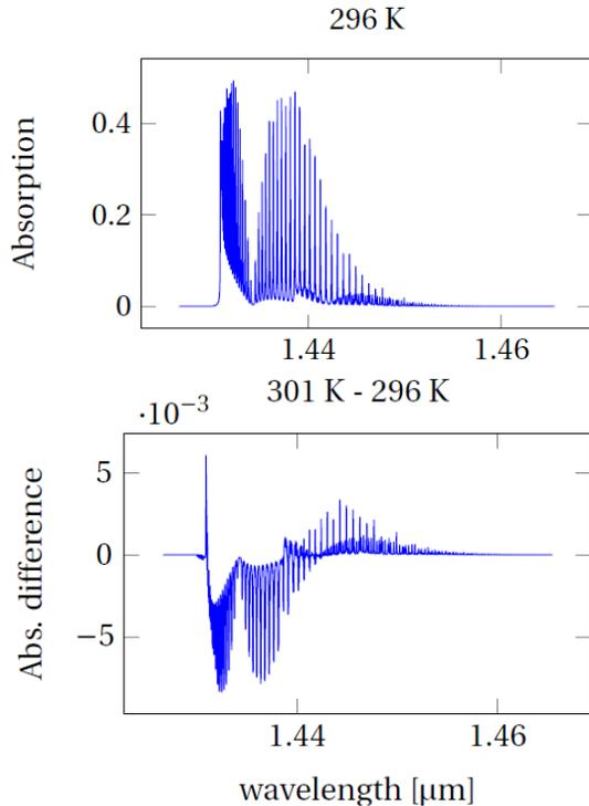
**Fig. 1** (top) Absorption spectrum after passing through 1.5 m of pure CO<sub>2</sub> at atmospheric pressure and a temperature of 296 K as obtained by HITRAN. (bottom) Difference in absorption for the same gas when changing the temperature to 301 K
