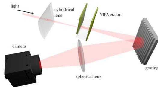
**Fig. 3** VIPA spectrometer consisting of VIPA etalon and a grating as pre-disperser.
