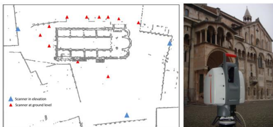
Fig. 2 The laser scanning survey of the cathedral of Modena: location map of the scanning positions (left) and a picture of the equipment, terrestrial laser scanner model Scan Station 2 by Leica Geosystems , during survey operations (right) (Castagnetti et al., 2012).
