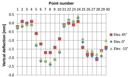
Fig. 2 Vertical deflections of the mast structure [2].
