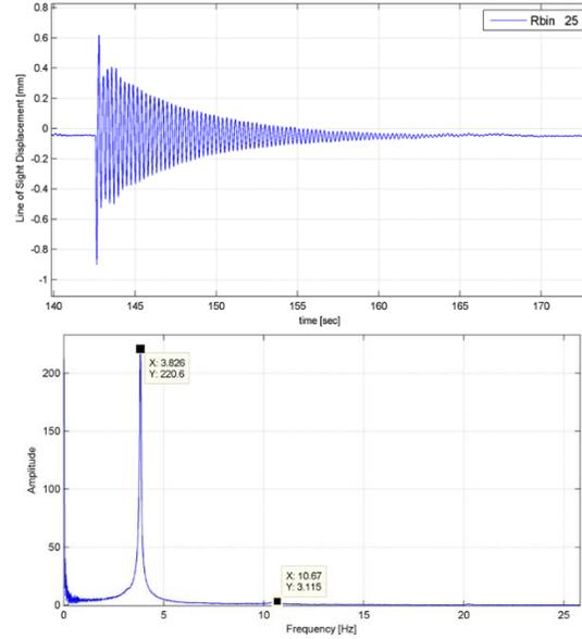
**Fig. 4** Example of time series based on line of sight displacement recorded by IBIS radar (upper) as well as corresponding FFT analysis (bottom).
