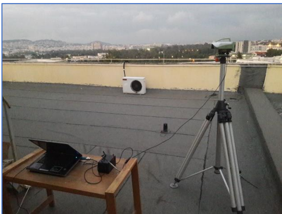
Figure 1. The automatic, stand alone and controlled set up of the DNA03 digital level.
