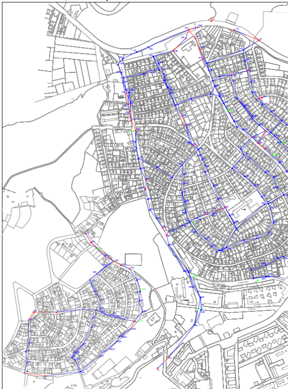
Figure 7. A part of the schema of the precise polygonometry and GNSS geodetic network
