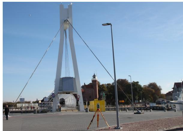
Figure 1. View of the footbridge and TS Leica TCRP 1201+ in the harbour scenery
