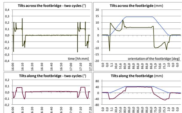
Figure 6. The graphs of two-axial inclinations of the footbridge during its opening and closing
