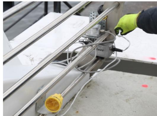
Figure 5. Inclinometer Posital AGS15 with counting device and the prism mounted at the end of the footbridge.
