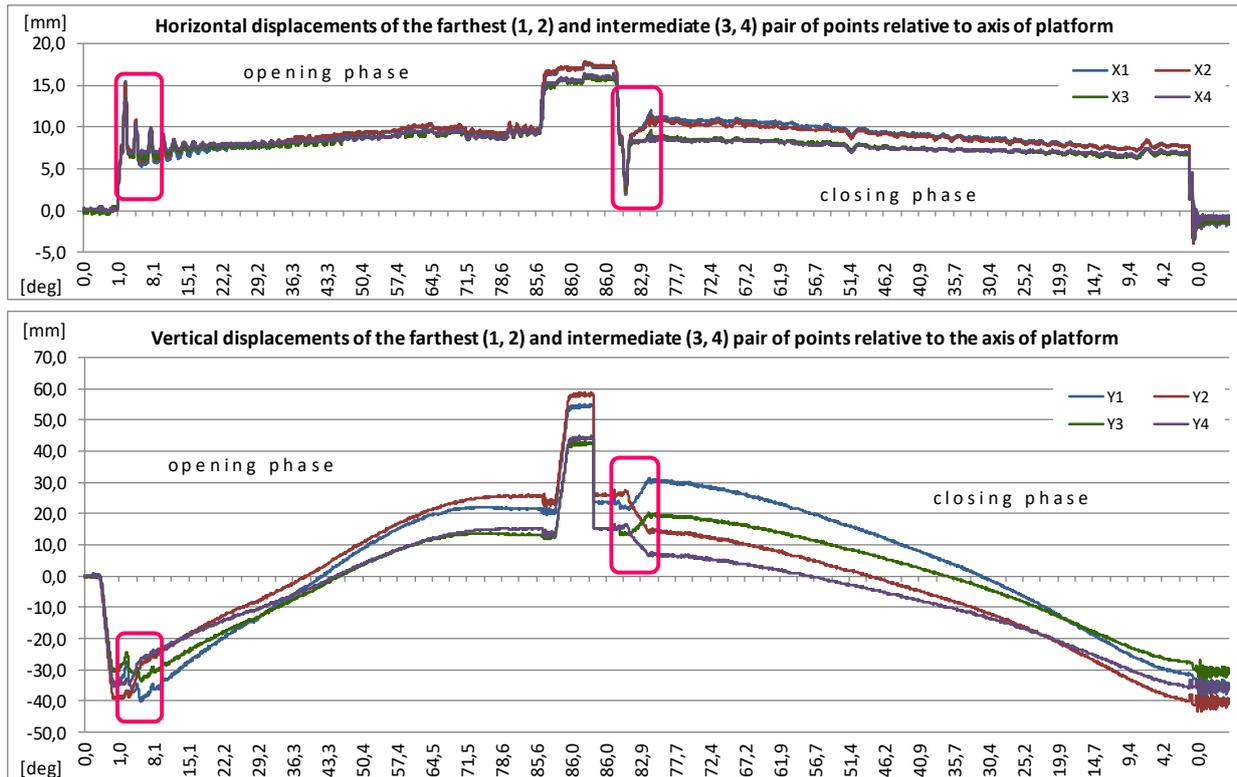
Figure 7. The graphs of horizontal and vertical vibrations recorded by high-speed camera
