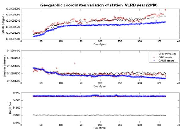
Figure 11. Comparison of time series obtained through SCRS-PPP, GINS and GAMIT/GLOBK softwares for a slow moving landslide at Villerville, France. (Boetzlé, 2015)
