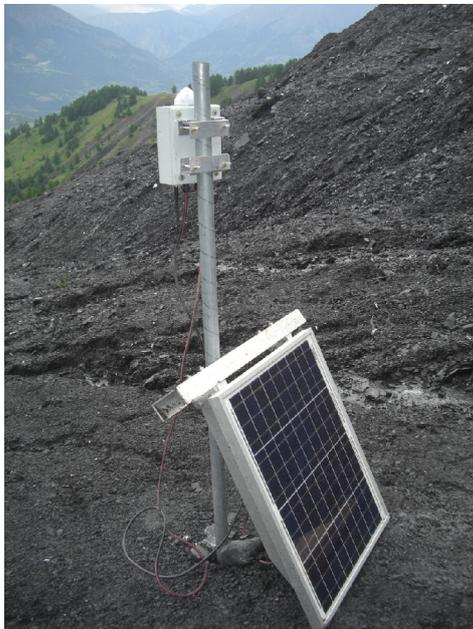
Figure 5. Geomon low-cost GNSS receiver and its solar panel on the Super-Sauze landslide (Boetzlé, 2015).
