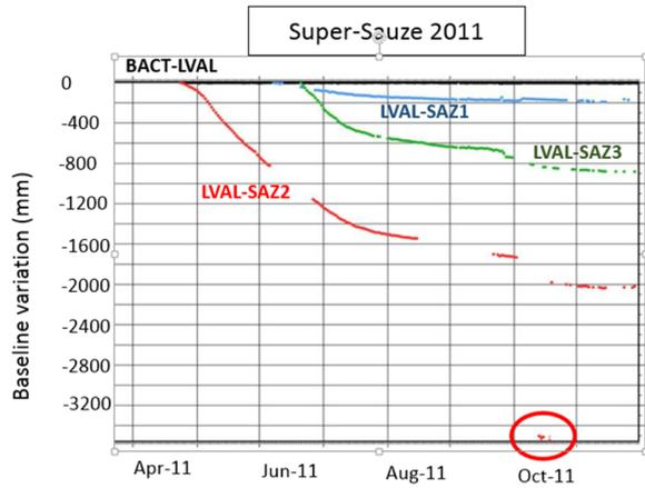
Figure 7. Example of anomalous estimation of baseline changes at Super-Sauze landslide (French Southern Alps) (Boetzlé, 2015).
