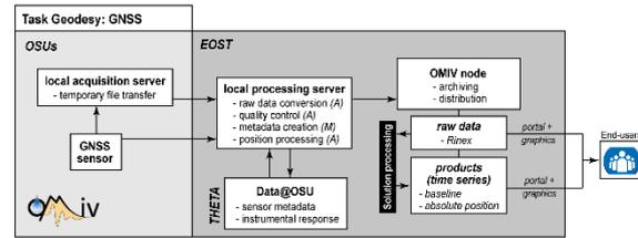
Figure 6. Global flowchart of GPS/GNSS data acquired at the French landslide Observatory OMIV (<http://ano-omiv.cnrs.fr>).
