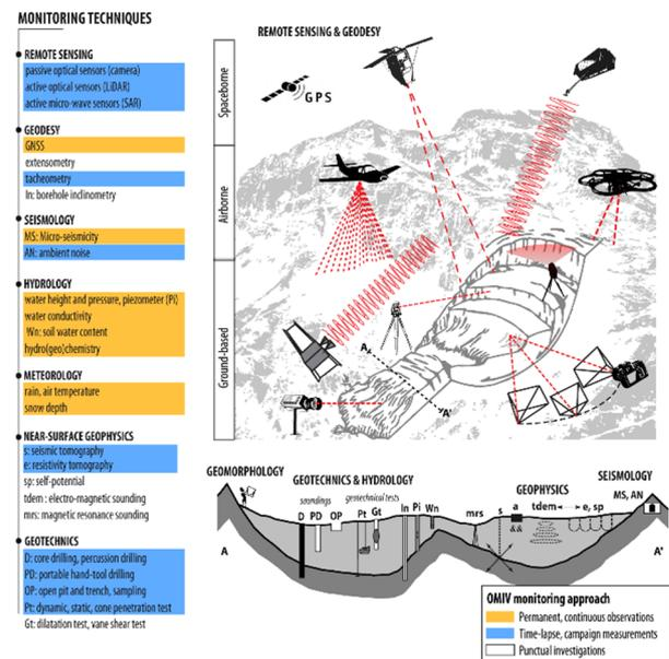
Figure 3. Multi-technique monitoring strategy at OMIV Landslide Observatory (<http://ano-omiv.cnrs.fr>).
