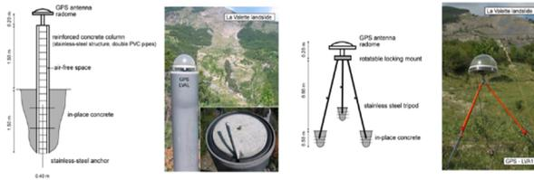
Figure 4. Permanent GNSS antenna on a pillar at the toe of La Valette landslide (Southern French Alps) and on-site GNSS antenna on the landslide. (<http://ano-omiv.cnrs.fr>).
