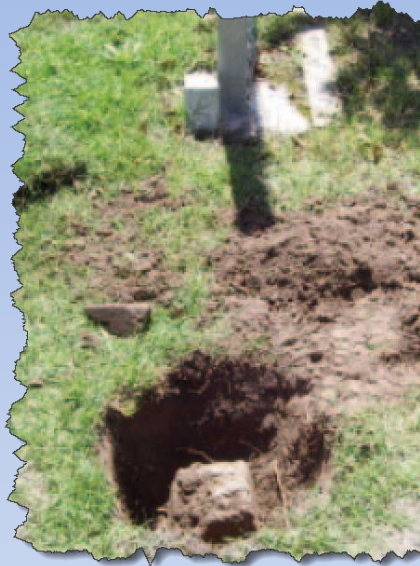
Concrete Block and Boundary Peg
