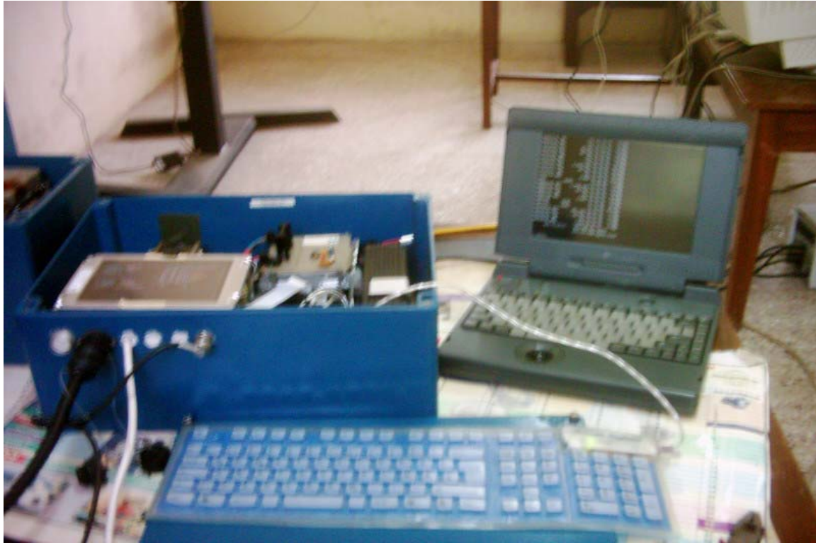
Fig. 3 GPS base station together with the computing and processing units.
