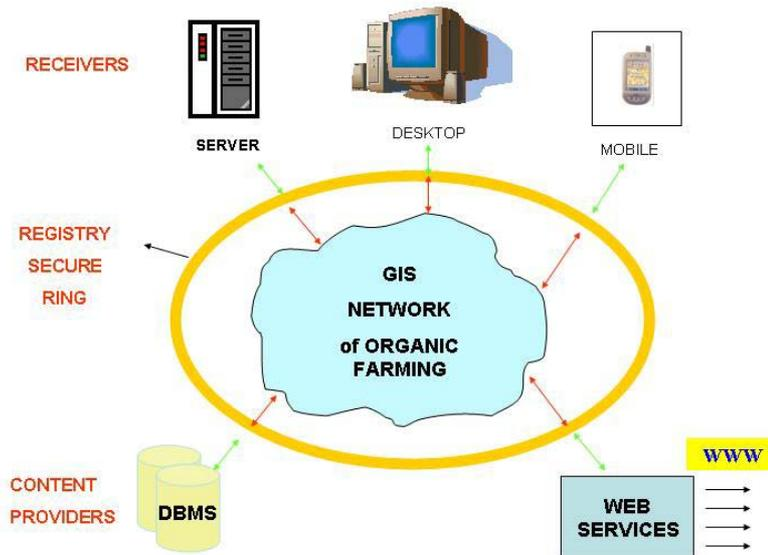
**Figure 4:** Components and Information Flow of a prototype Web based GIS system with a secure ring where needed.
