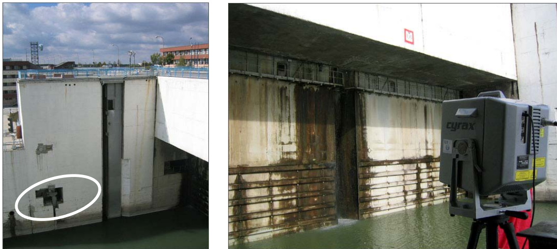
Fig. 3: TLS station during the gate measurement
