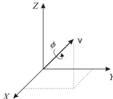
**Fig. 2:** Geometrical Interpretation of a Rotation Quaternion
