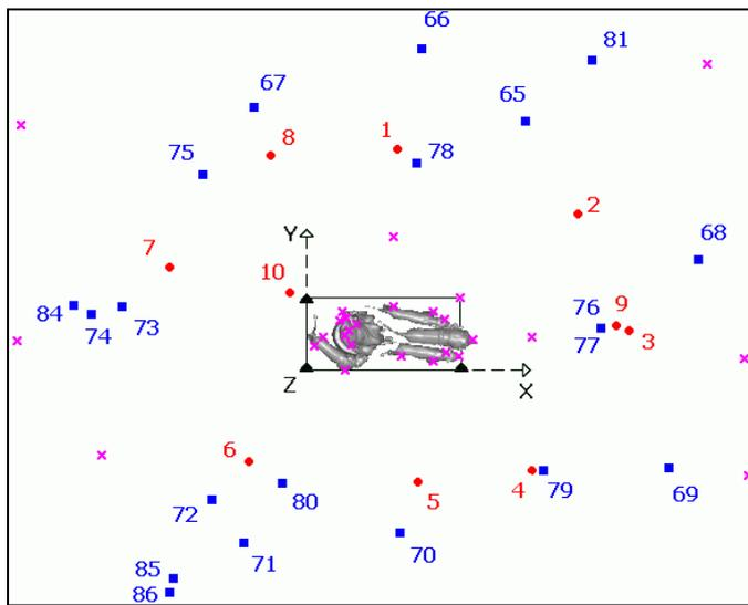
**Figure 3:** Configuration of the 20 scan (red circles) and 22 camera (blue squares)-positions
