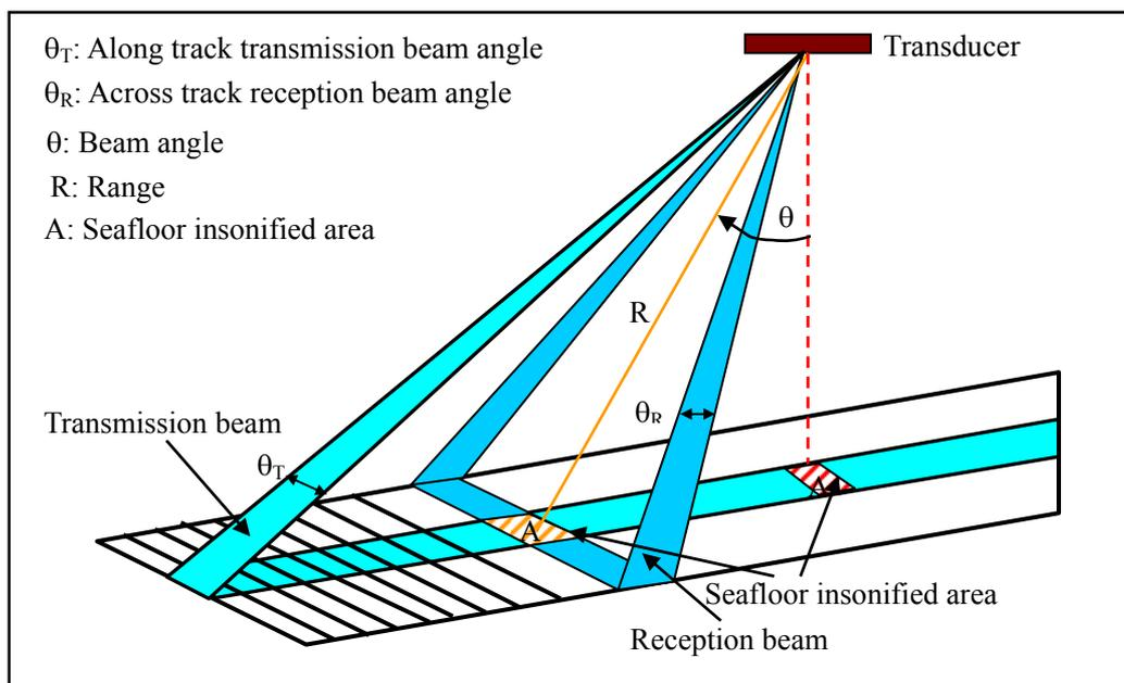
**Figure 1.** Beam geometrical configuration of multibeam echo sounder
