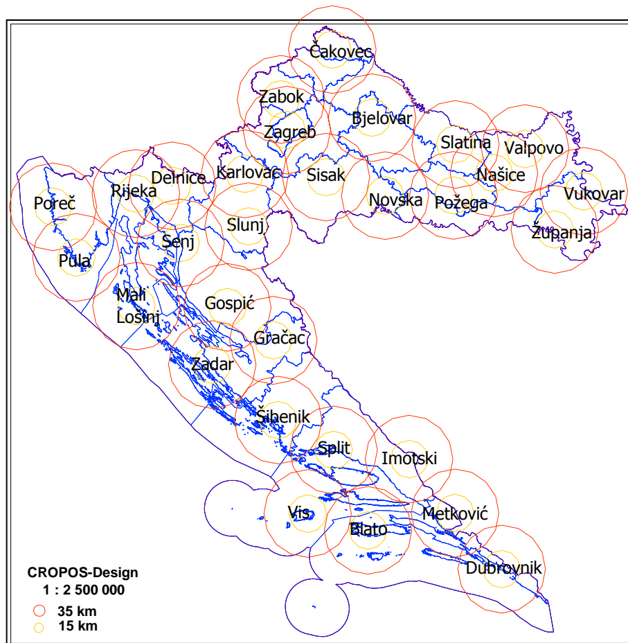
Fig. 4: Design of the CROPOS system
