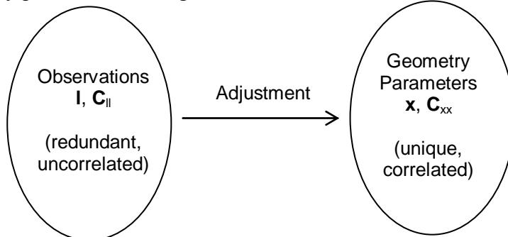
Figure 5-1: Mapping of Observations onto Unique Geometry Parameters
