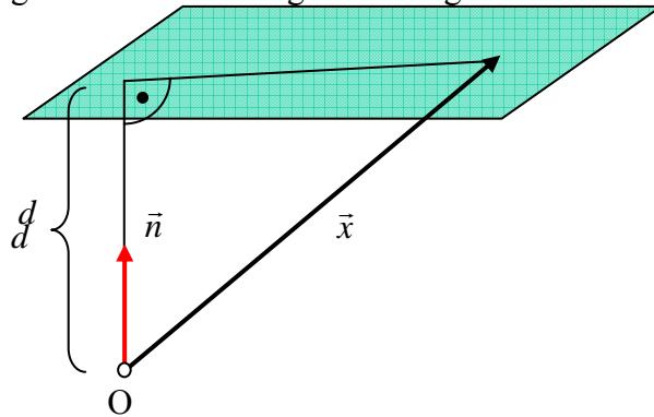
**Figure 4-2:** Geometrical Illustration of a Plane Equation
