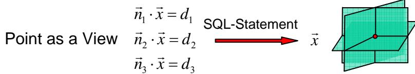
**Figure 4-4:** Point Coordinates as View on Plane Parameters
