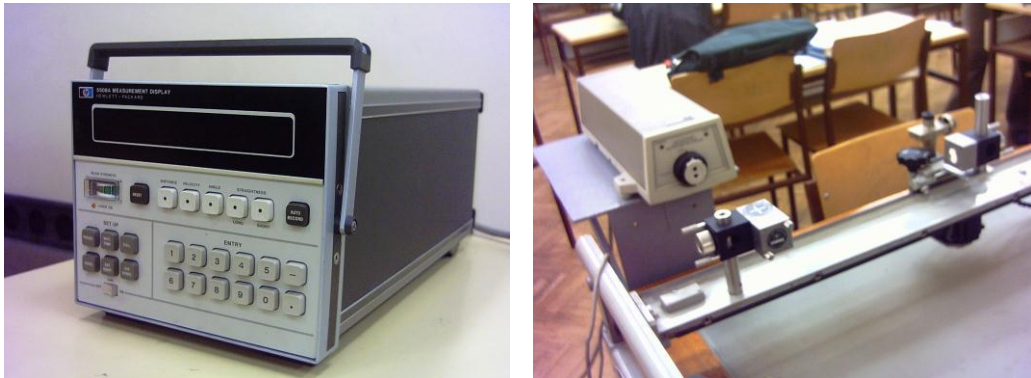
Picture 1: Laser interferometer system HP 5528A
