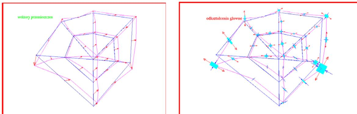
**Fig. 6.** Dislocation vectors and coordinates of the tensors of main strains
