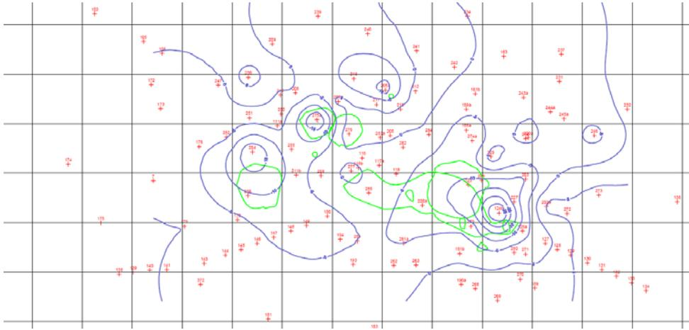
**Fig 4.** Isoclines of subsidence speed in the period between May and November 2001.
