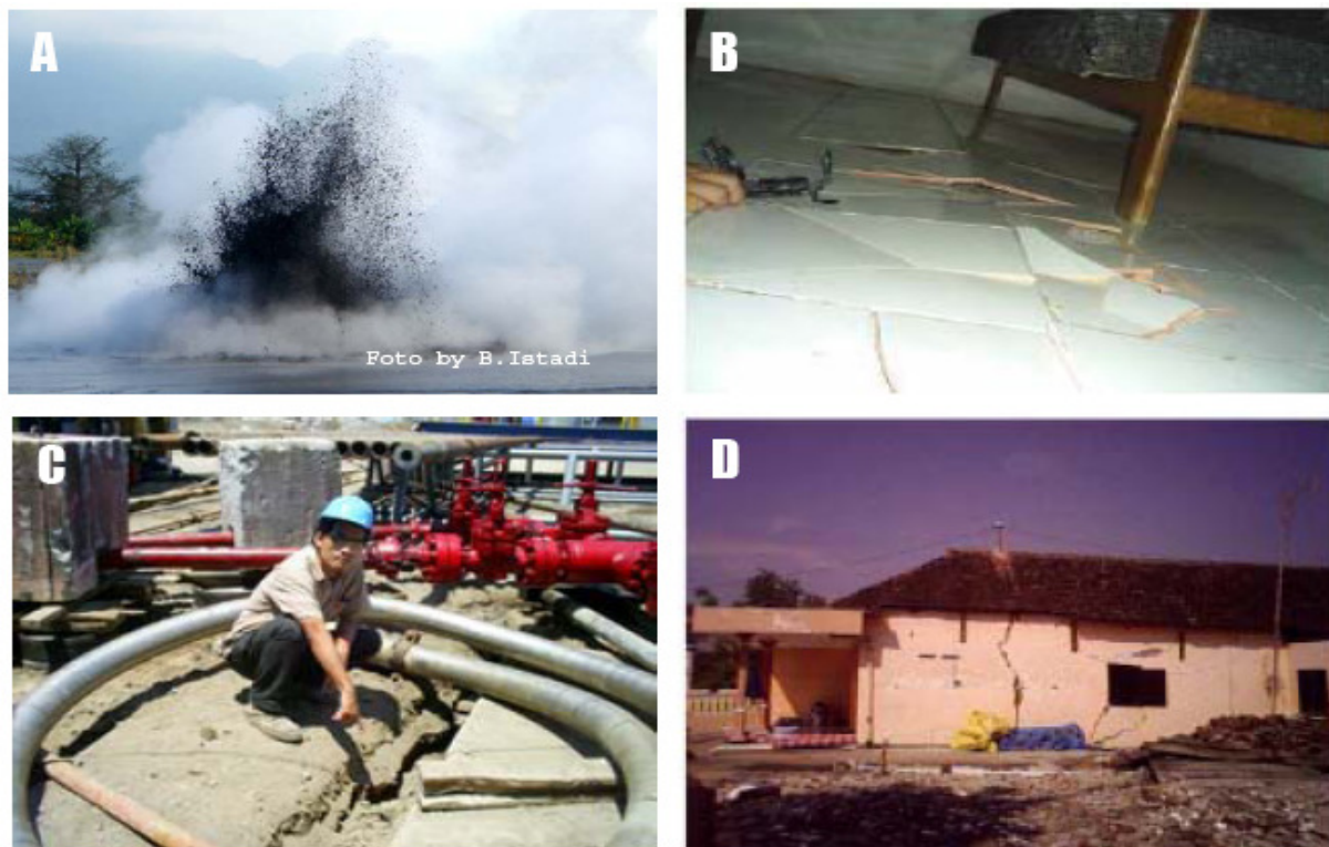
Figure 1 (a) LUSI mud volcano eruption, (b) crack on the floor, (c) cracks on the ground around relief well 1, (d) crack on the house in Sengon Village.
