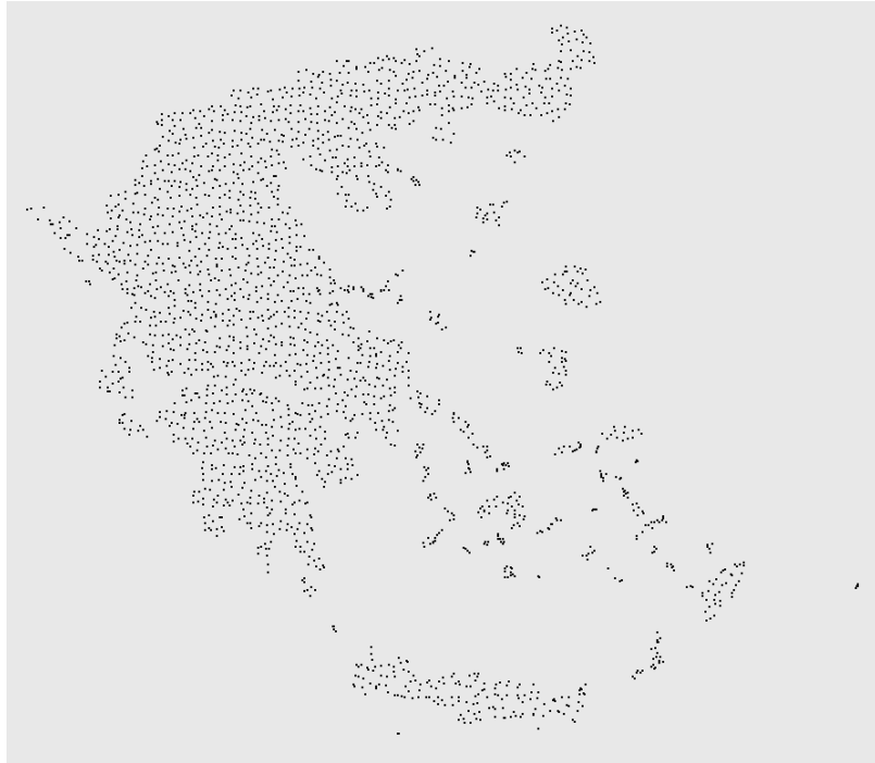
Figure 2: The 2470 trigonometric points measured for the computation of transformation parameters.
