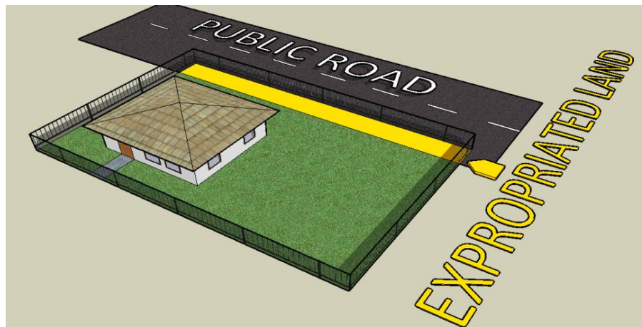
Fig.2. Visualisation of a partial property expropriation example for widening a road - Scenario 1
