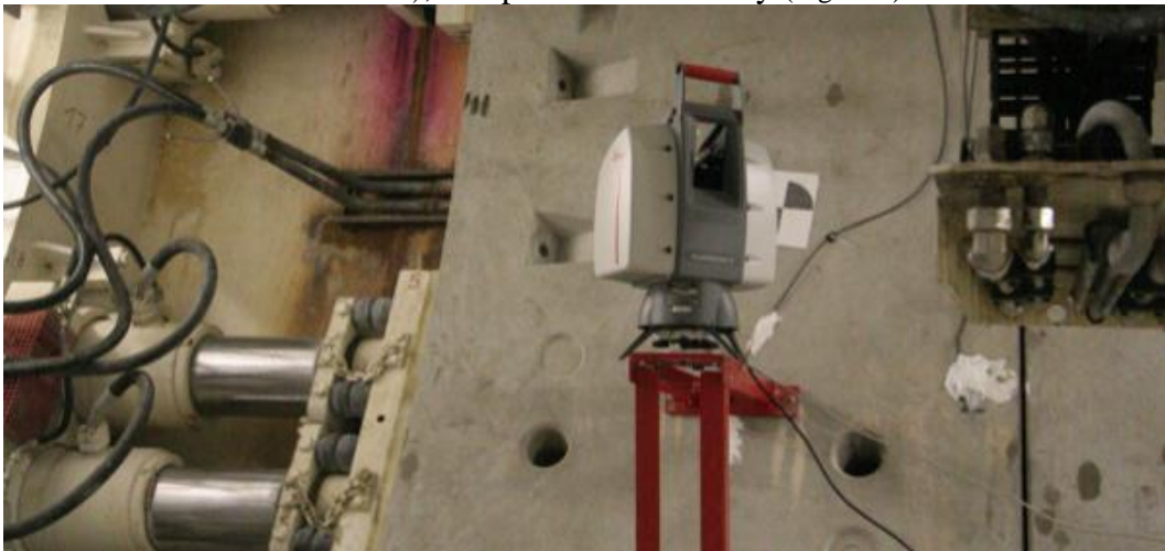
Figure 5: Laser scanner mounted on a tunnel bracket attached to the concrete tunnel section (Source: A. De Wulf, 2009)
