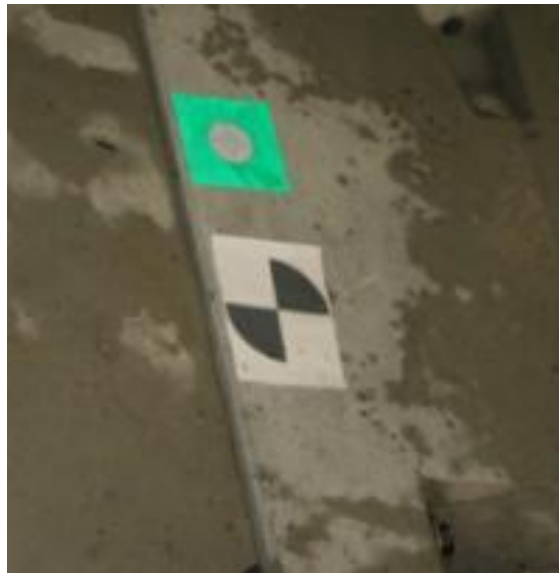
Figure 6: Trimble Target (Upper example) - Leica Target (Lower example) (Source: A. De Wulf, 2009)
