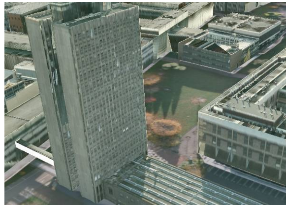
Figure 5. 3D building models merged with the terrain model, ortho-images and building texturing of the University Park campus
