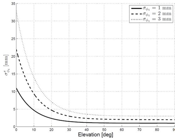
Figure 2: Elevation dependent weighting function for different values of coefficient  $\sigma_{\phi_i}$
