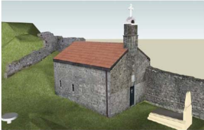
3D model of the church at Medun (near Podgorica) generated from the data from laser scanning and digital photogrammetry
