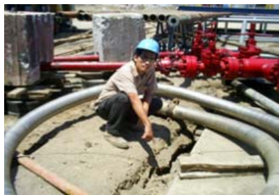
Crack on the ground around Relief Well 2.
