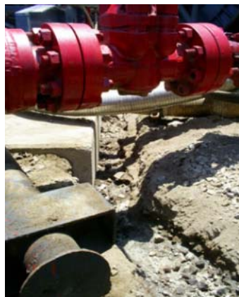
Crack on the ground around Relief Well 2.
