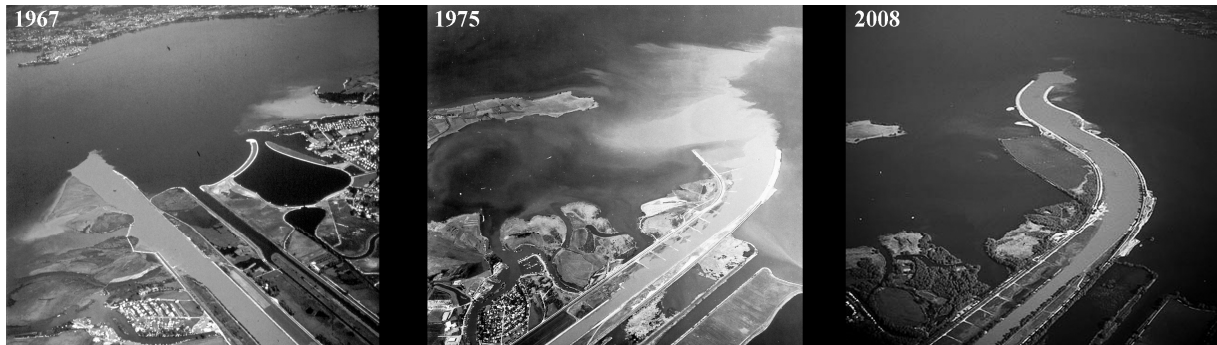
Figure 1: Sedimentation process and the subsequently undertaken embankment dam constructions at the Rhine delta ()
