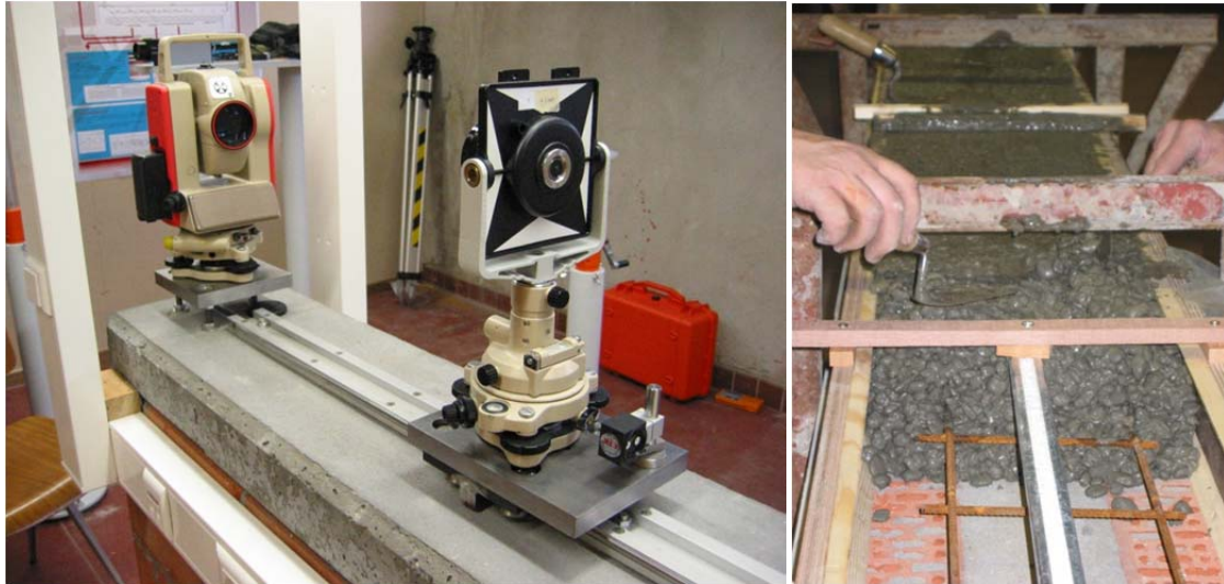
Figure 2: Movable carrier and EDM total station (left) and construction of the calibration bench (right)
