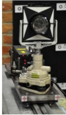
Figure 8: Movable carrier with two targets on the base plate under the tri-branch
