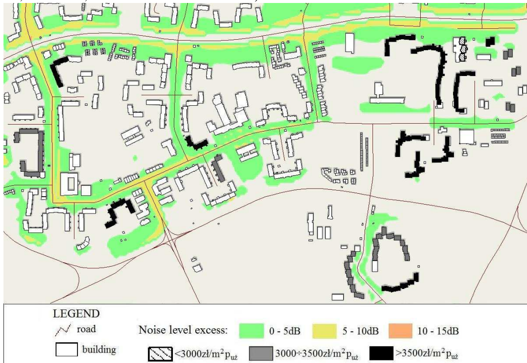
Graph 3. Spatial location of apartment transactions in relation to a map of excess road traffic noise L_{DWN} (Przylesie, Bohaterów, Akademickie-Wschód districts)
