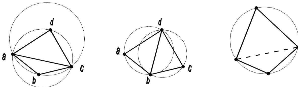
Figure 1: Delaunay triangle principle
