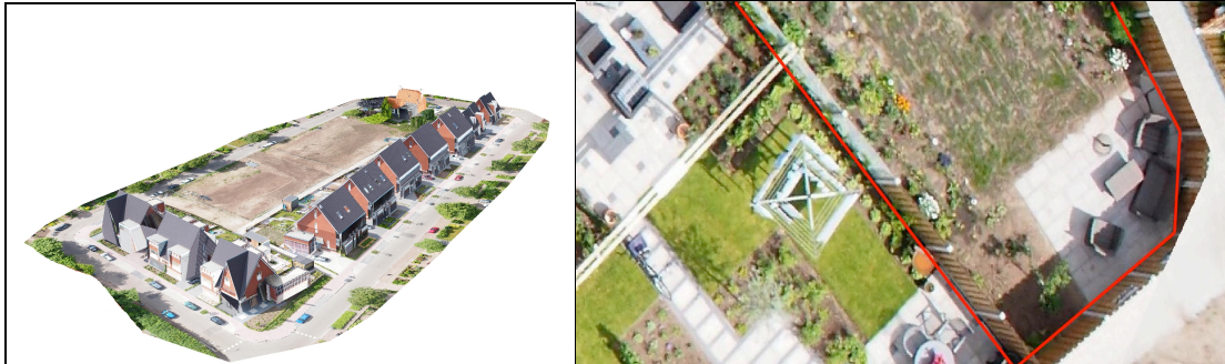
Figure 3 and 4: Automatic DTM creation and zoomed-in orthophoto made by PIX4UAV with cadastral borders.
