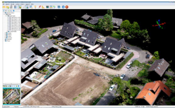
Figure 7: 3D pointclouds extracted from high resolution aerial (UAV) dataset.
