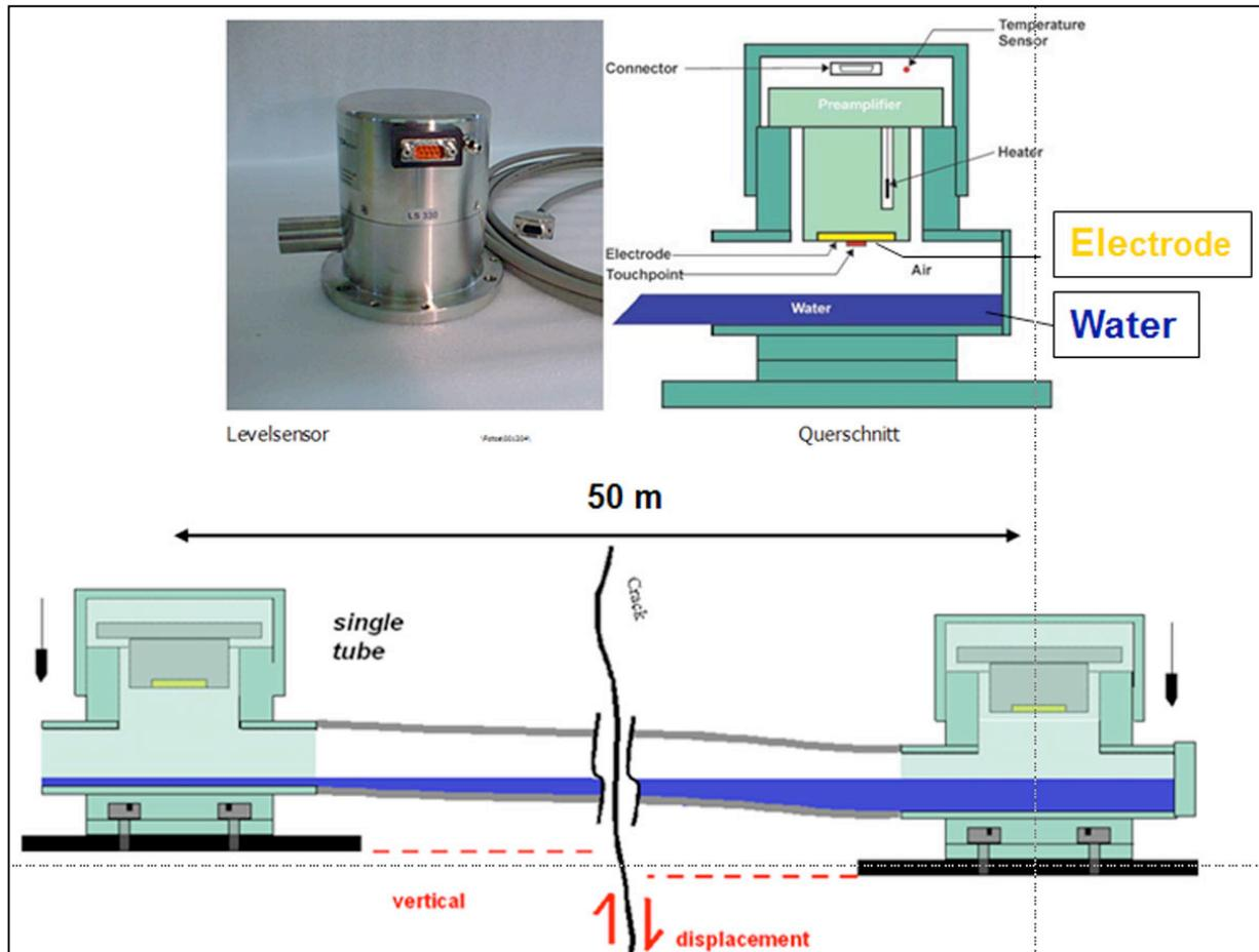
Fig. 3): HLS measuring principle
