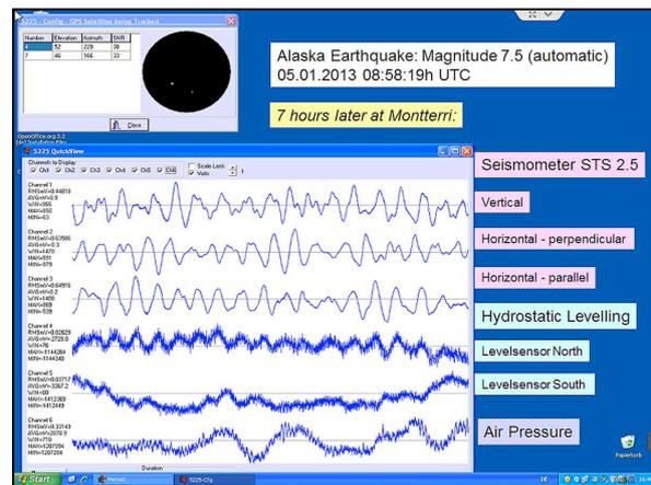
**Fig. 13):** Alaska Earthquake, 05.01.2013 08:58:19 h, recorded 7 hours later; additional air pressure channel. The time window is 120 sec. The dominant period is now 7 sec, the marine microseisms, which is visible also at HLS.
