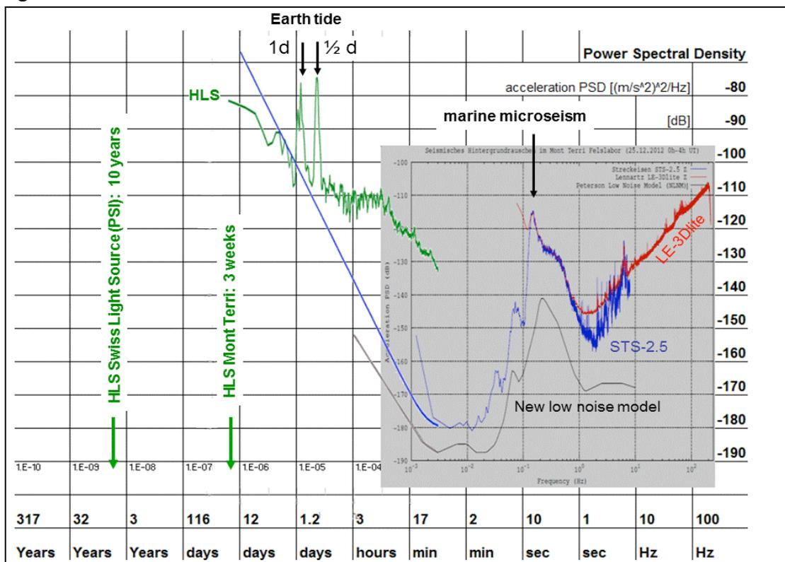
Fig. 14): Seismic background noise expanded with HLS Signal
