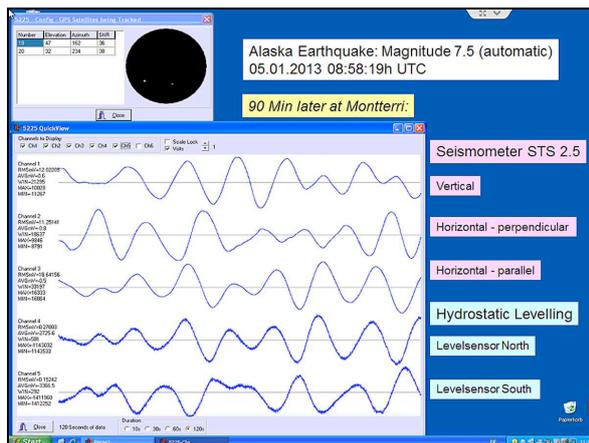
**Fig. 12):** Alaska Earthquake, 05.01.2013 08:58:19 h, recorded 90 min later at Mont Terri. The time window is 120 sec. The dominant period of the waves is about 30 sec
