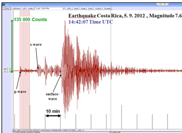
**Fig. 8):** Costa Rica Earthquake, 5 September 2012, magnitude 7.6, recorded at Mont Terri rock laboratory. Plot scale 135 000 counts
