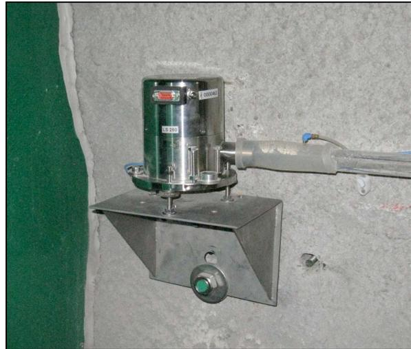
**Fig. 7):** HLS sensor North on stainless steel console mounted with 2 one meter long M20 threaded rods
