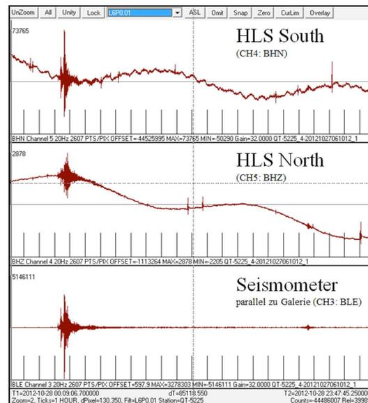
Fig. 11): Masset Canada Earthquake, HLS and seismometer one day record
