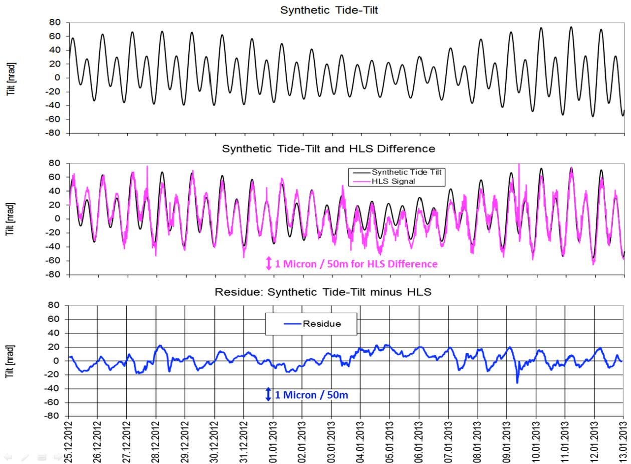
**Fig. 15):** Superposition of synthetic tide-tilt and HLS results (shifted) and difference plot
