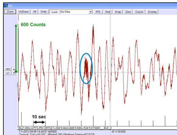
**Fig. 9):** Microseismic noise, shortly before the Costa Rica Earthquake from 5 September 2012. Plot scale 600 counts
